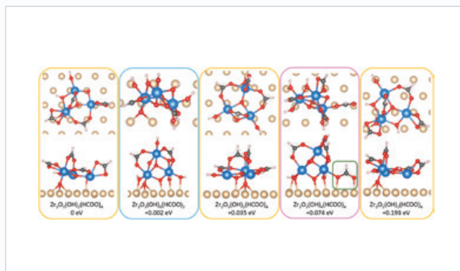
Catalyst configurations with lowest free energy from each defined family and metastable structures that dominate the catalytic activity. Image: Yang et al. J. Am. Chem. Soc. 2025, 147, 18, 15294–15306
