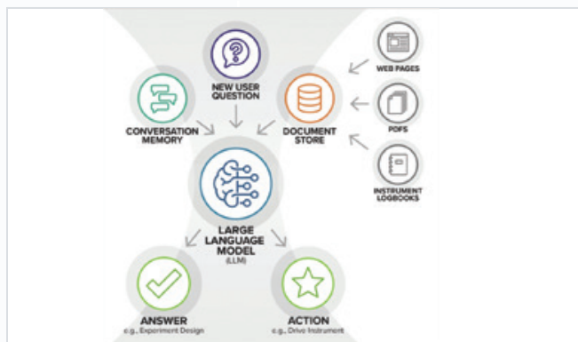
Overview of CALMS: CALMS uses a large language model in conjunction with conversational memory, document stores, and experimental tools to answer user queries or take action to drive an instrument. Image: Prince et al. npj Computational Materials 10, 251 (2024).
