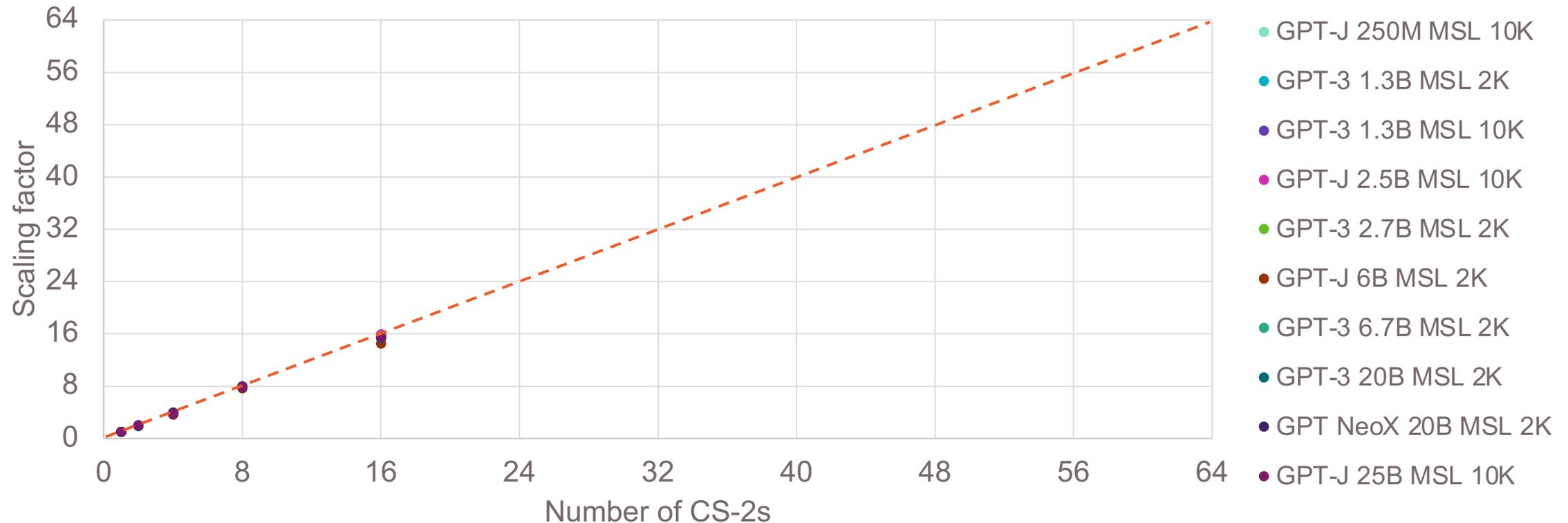
**Figure.** Measured training throughput scaling for 250M-20B GPT models over 1-16 CS-2 systems; projected scaling to 64 systems.
