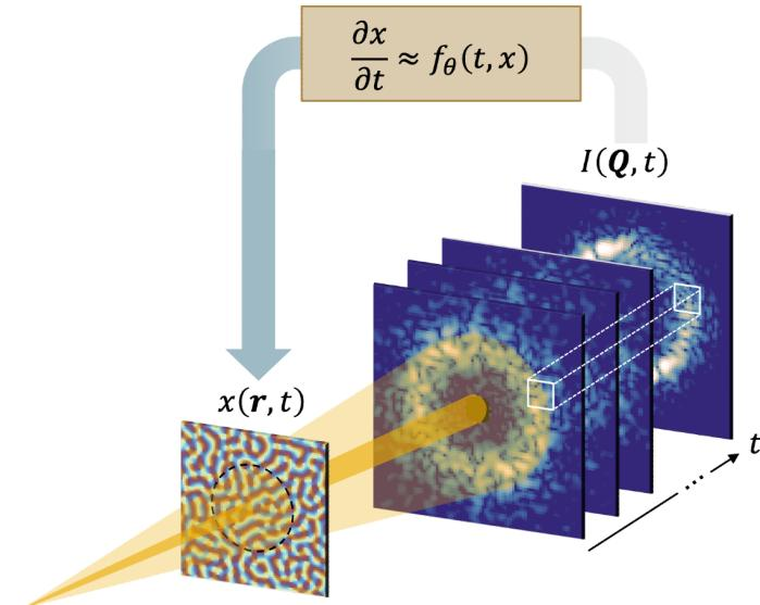
Data-driven discovery of materials' dynamics from coherent scattering
