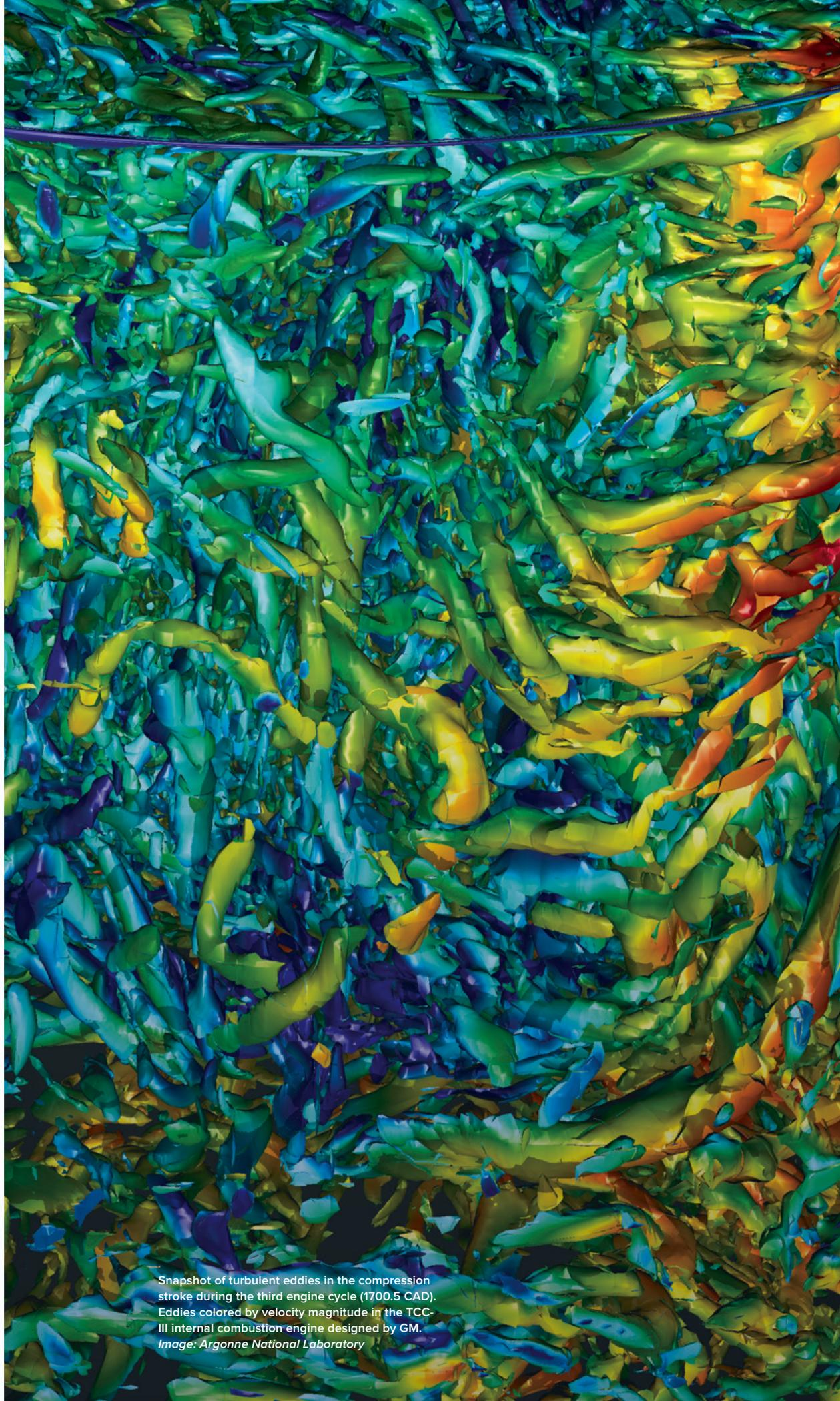
Snapshot of turbulent eddies in the compression stroke during the third engine cycle (1700.5 CAD). Eddies colored by velocity magnitude in the TCC-III internal combustion engine designed by GM.
