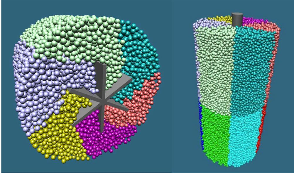
Figure C.8 These simulation images show suspended particles in a 6-blade rheometer for NIST’s proposed mortar Standard Reference Materials (SRM). The spheres, which are color-coded by their starting location in the rheometer, are suspended in a cement paste with properties derived from NIST’s cement paste SRM.
