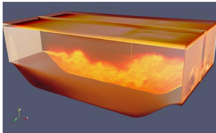
Figure 4.1 Periodic Hill Generated by OpenFOAM
